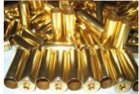
Dirty Brass + Cleaning Media from Walmart+ Stainless Steel Pin Media tumbled for 4 hours in a Thumler's High Speed Model B produces the bling shown in the bottom picture. Impressive!
